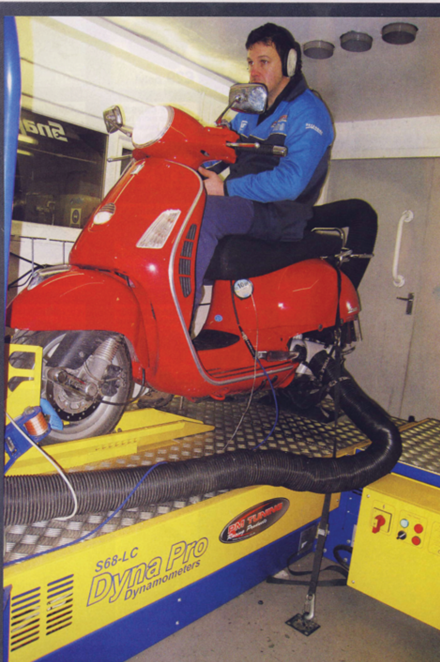
PM Tuning use a Dyna Pro eddy current dyno to load the GTS for testing. Paul's test technique is very thorough and scientific.
